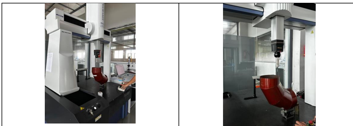
Fig. 2. Verification of Dimensions using coordinate measuring machine (CMM)
