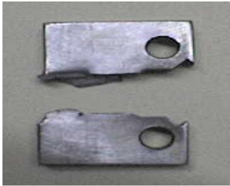
“Figure 3. Specimen before fatigue failure and after failure”
