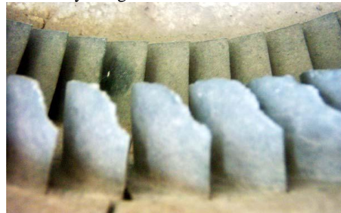
Fig 1.2: Failed Stator Blades
