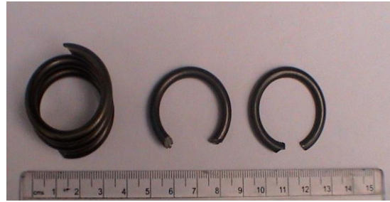
Fig.2 Broken Engine valve spring
