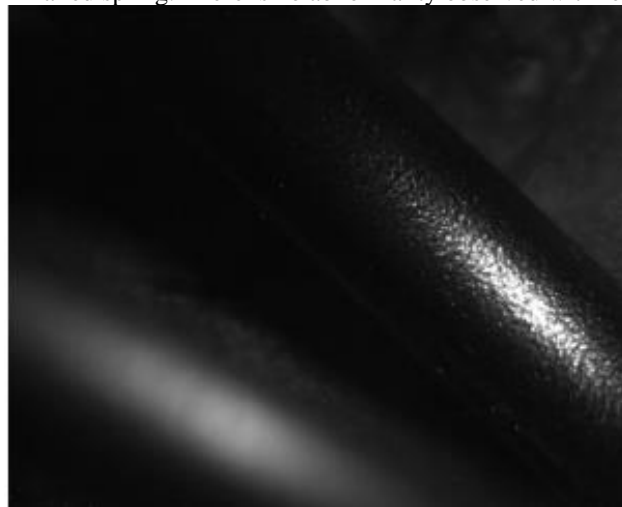
Fig.14.Good shot peening coverage on failed spring
