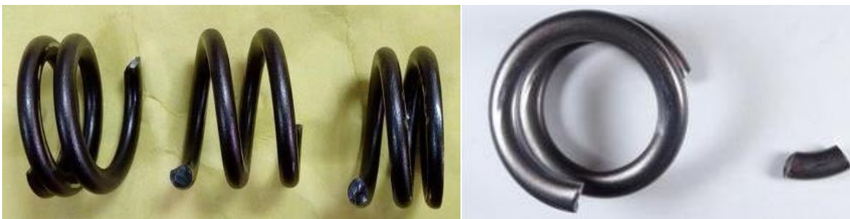
Fig. 1 and 2. The broken exhaust valve spring in the diesel engine and multiple fracture faces
