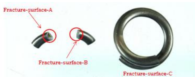
Fig.3. Fracture faces removed from the failed spring
