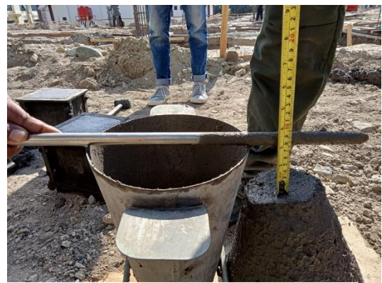
Figure 13. Concrete slump testing
