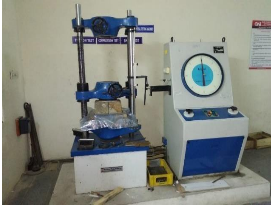
Figure 2.1 Compression of Fibre Laminates on UTM
