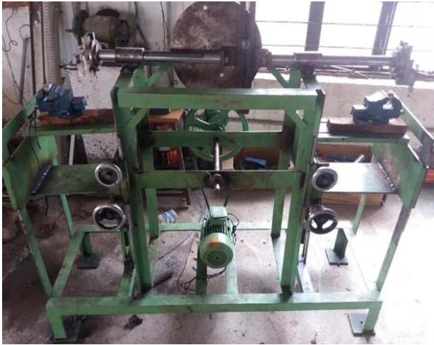
Fig:- Proto type of dual side shaper machine
