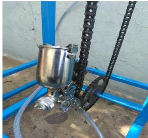
Fig. 4: Spray Gun Setup
