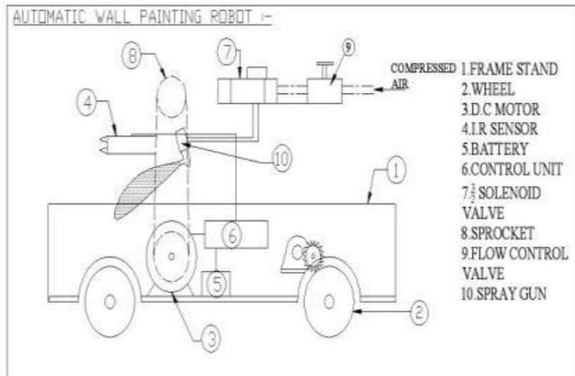
Fig.1: Block diagram of Automatic Wall Painting Machine
