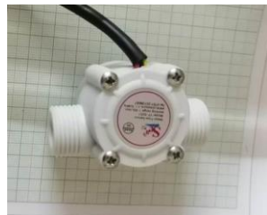
Fig.3.3 Water flow meter
