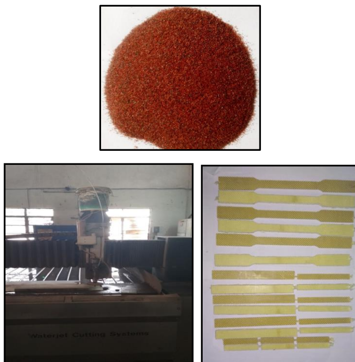
Figure 3: Garnet sand (abrasive), water jet cutting, cut specimens.
