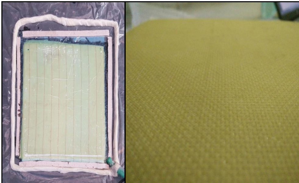
Figure 2: Vacuum resin transfer molding and Fabricated material
