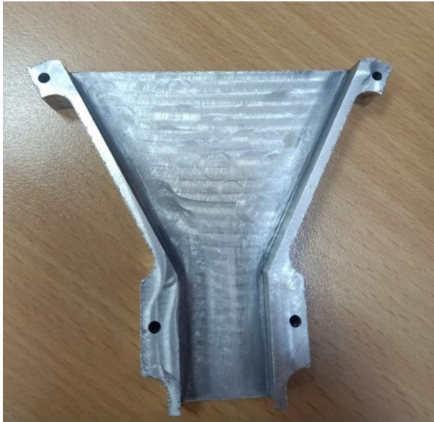
Fig. 8. A piece of the base plate of the horn antenna
