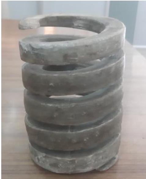
Fig. 2 Fabricated GI/Ep/Ceno FRP helical spring
