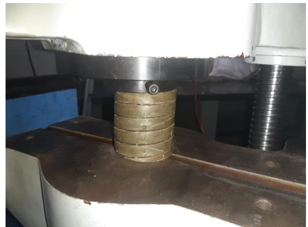
Fig. 4 Solid length of GI/Ep/Ceno FRP-Helical spring
