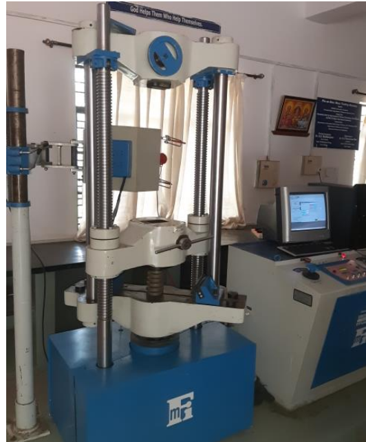
Fig. 3 testing of fabricated GI/Ep/Ceno FRP helical spring on UTM
