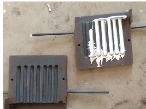
Figure 2.4 Cast Iron Die and Composite samples
