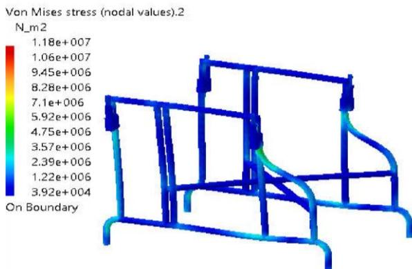
Fig. 8 Stress on Base Structure at 80 kg Test Load
