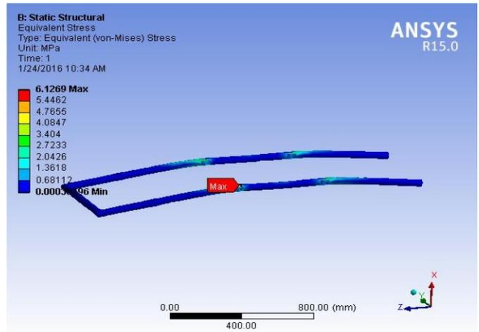
Fig. 5 Stress on Links at 65 kg Test Load
