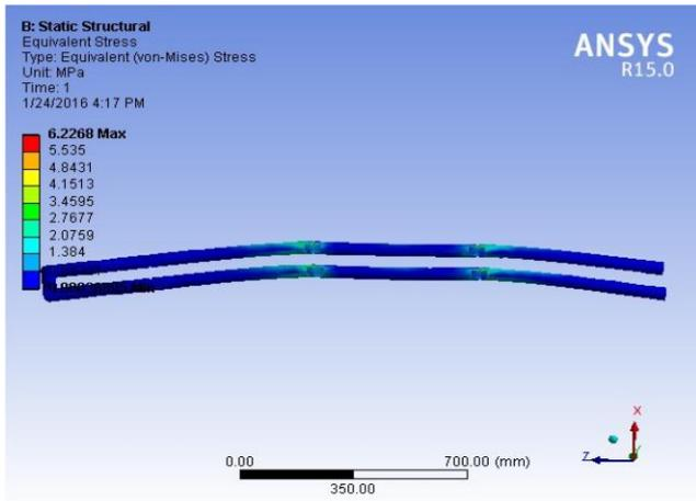
Fig. 7 Stress on Links at 70 kg Test Load
