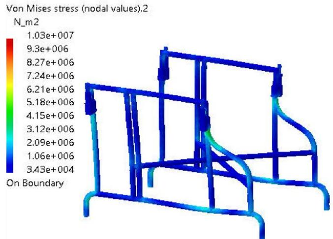
Fig. 6 Stress on Base Structure at 70 kg Test Load
