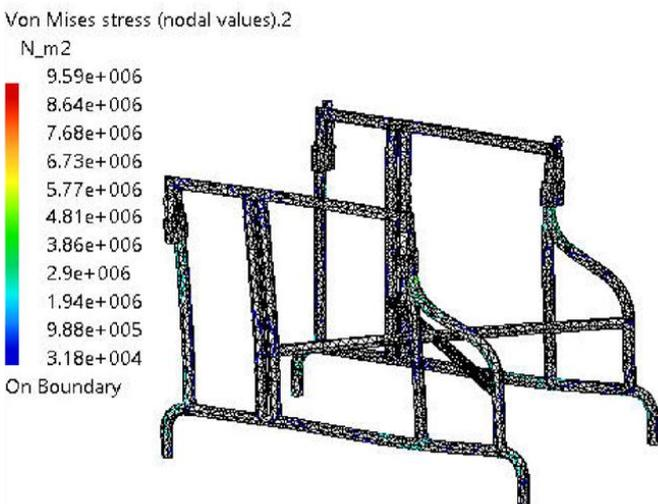
Fig. 4 Stress on Base Structure at 65 kg Test Load
