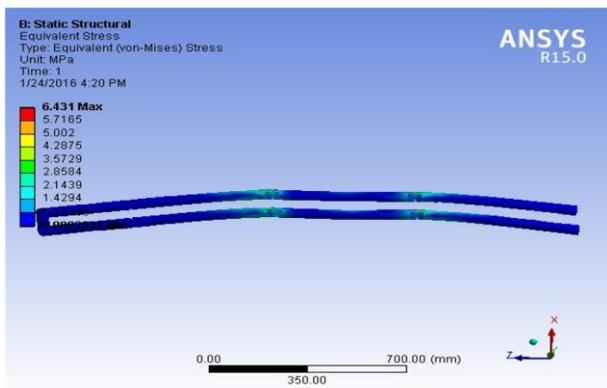
Fig. 9 Stress on Links at 80 kg Test Load
