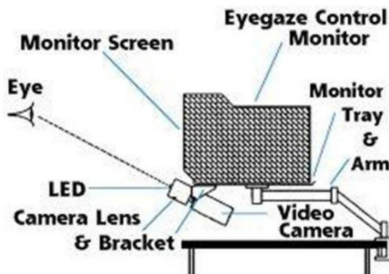
A user operates the eyegaze System by looking at rectangular keys that are displayed on the control screen. To "press" an eyegaze key, the user looks at the key for a specified period of time. The gaze duration required to visually activate a key, typically a fraction of a second, is adjustable. An array of menu keys and exit keys allow the user to navigate around the eyegaze programs independently.
