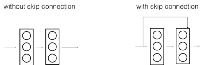
Fig. 6. Resnet skip connection
