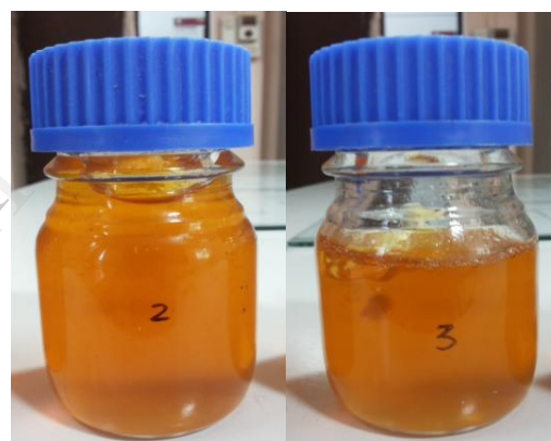
Fig.8 Jelly developed by adding SLPP pectin extracted by using citric (3) and nitric acid (2)
