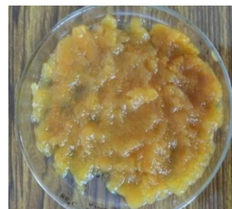
Palate 4. Refined pectin after centrifuge
