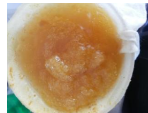
Palate 3. Coagulated pectin after ethanol addition and strained after refrigeration
