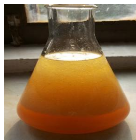
Palate 3. Coagulated pectin after ethanol addition and strained after refrigeration
