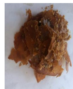
Palate 5. Dried pectin extracted using citric and nitric acid
