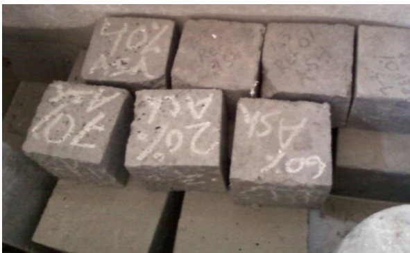
Fig.3.2 concrete cube specimens with and without replacement level
