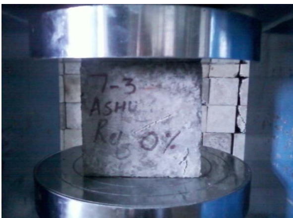
Fig.3.3 test setup of cube specimen
