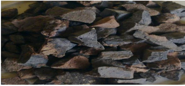
Fig.2.1 Typical shapes of Over Burnt Aggregate
