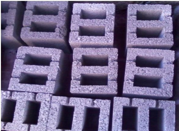
Fig.3.1 concrete hollow blocks with Different percentage of OBA
