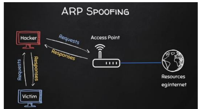
Fig. 3. Pictorial demonstration of ARP spoofing
