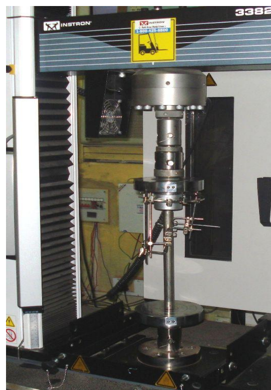
Fig. 3: JESS specimen under axial compression on universal testing machine
