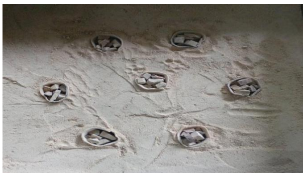
Fig. 5. Group encased column
