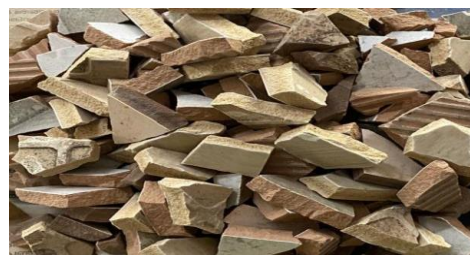
Fig. 2. Broken Tile Waste.
