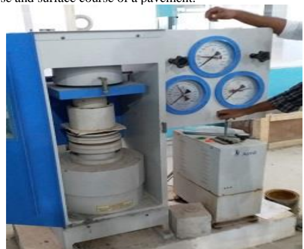
Fig. 2 Test setup for crushing value test
