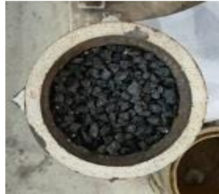
Fig. 1 Electric arc furnace slag
