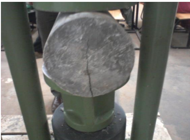
TESTING COMPRESSION CYLINDER
