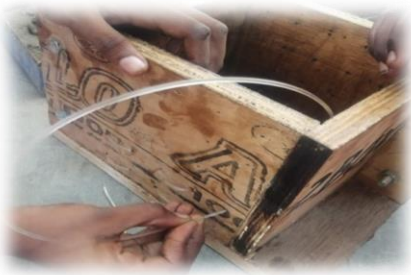
figure1.1 placing of fibre
