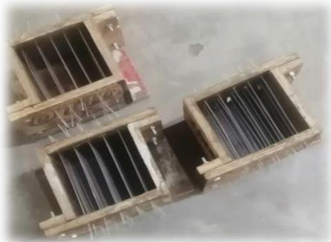
fig.1.2. mould after placing of optical fibre.
