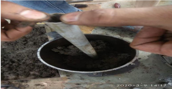
Fig 4 Stone column casting
