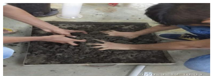
Fig 2 Mixing of soil sample at OMC
