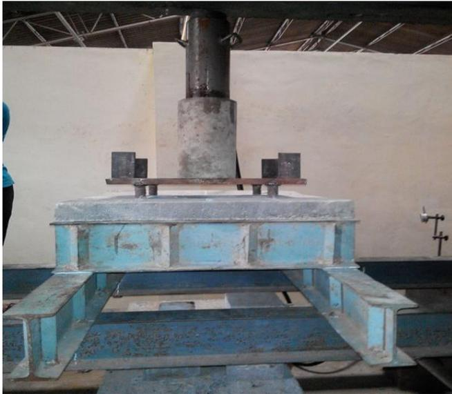
Figure 1.3: Flexural test setup
