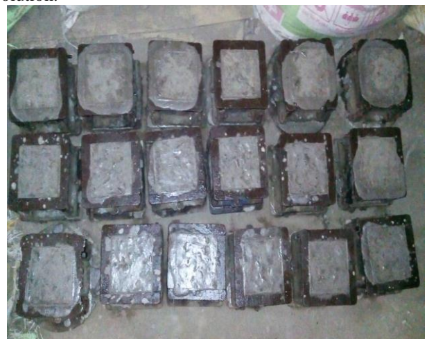
Figure.2 casting of specimens
