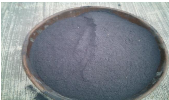
Figure.1 RHA after grinding
