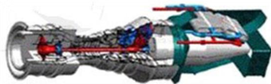
Fig. 1. The recuperative engine. The heat exchangers are installed in the exhaust nozzle.
