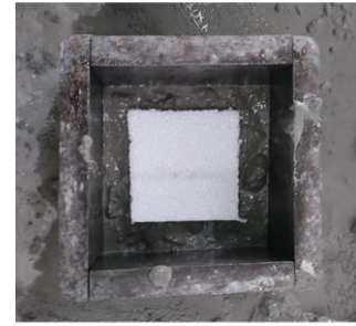
Figure 3: Mold for casting concrete blocks
