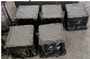
Figure2: Casting of Blocks (150mmX150mmX150mm)
