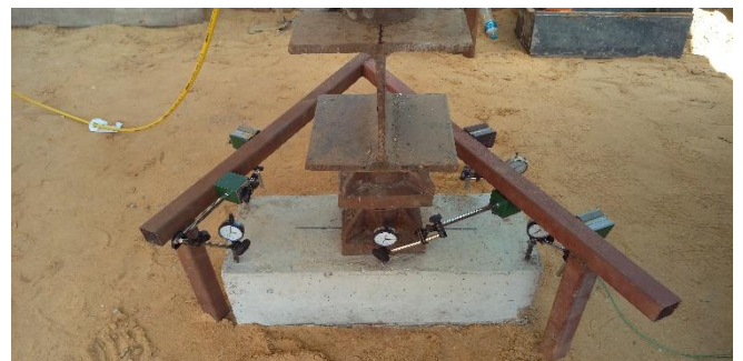
Fig. [17] Loading Jack and Dial Gauges Setup for Group (2) – Group of Two Piles
