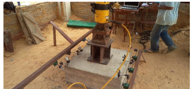
Fig. [23] Loading Jack and Dial Gauges Setup for Group (4) – Group of Four Piles
