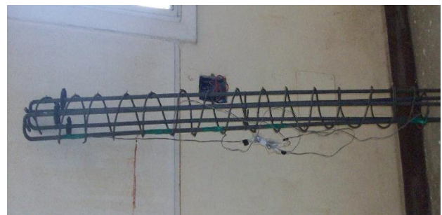
Fig. [5] Internal Strain Gauges
