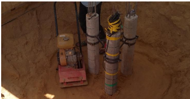
Fig. [19] Placing Compacted Soil around Tested Pile Groups for group (3) – Group of Three Piles
