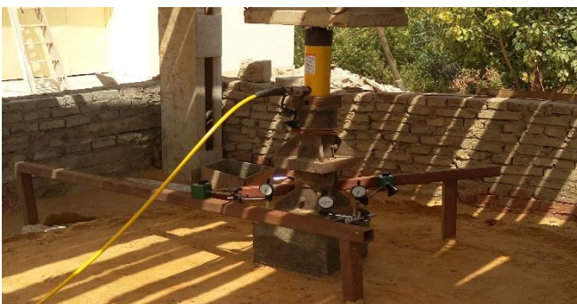
Fig. [14] Loading Jack and Dial Gauges Setup for Group (1) – Single Pile
