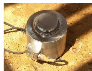
Fig. [10] Load Cell
