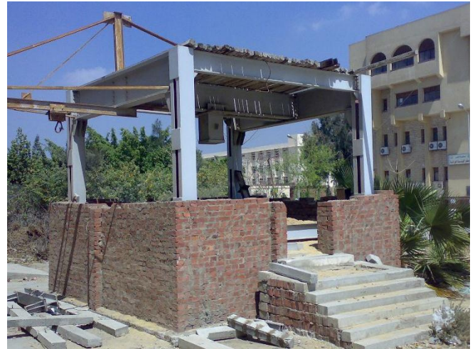
Fig. [8] Loading Frame
