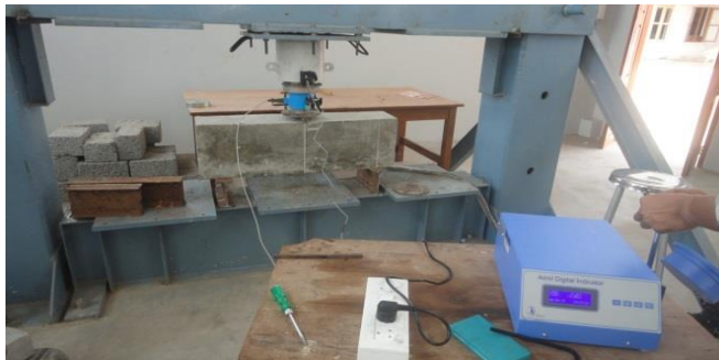
Fig.7. Experimental Setup of Beam Specimens
