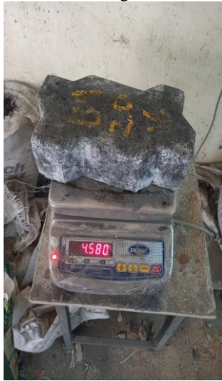
Fig. 10 – WATER ABSORPTION TEST
