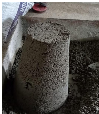
Fig. 6 – SLUMP CONE TEST
