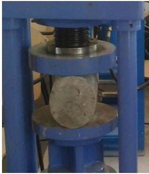
Fig 2. Split tensile strength test
