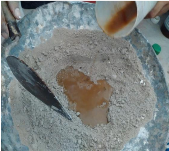
Figure 1: preparation of pozzolanic lime mortar
