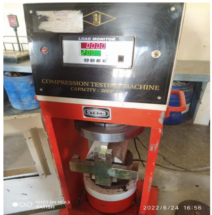
Fig. 4. Split tensile strength testing
