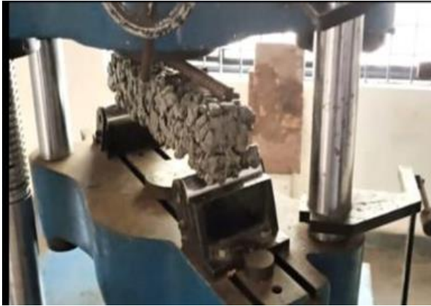
Fig 3.3 Flexural strength testing on UTM
