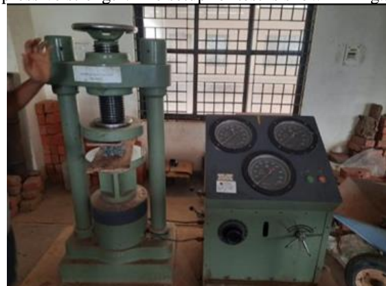
Fig 3.2 Compressive strength testing on compression testing machine
