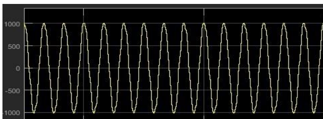
Figure 13. Load current waveform with no filters connected to load 2
