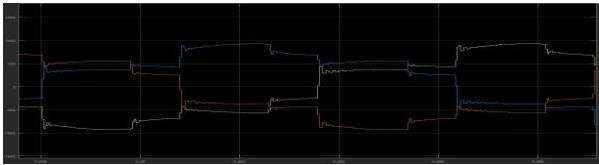
Figure 12 Load voltage with no filters connected to Load 1
