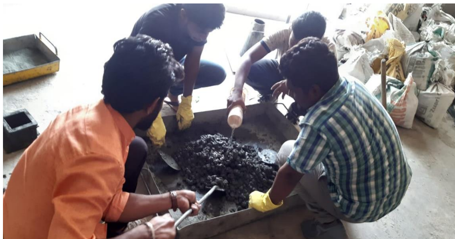
Fig.1 Polymer concrete mixing
