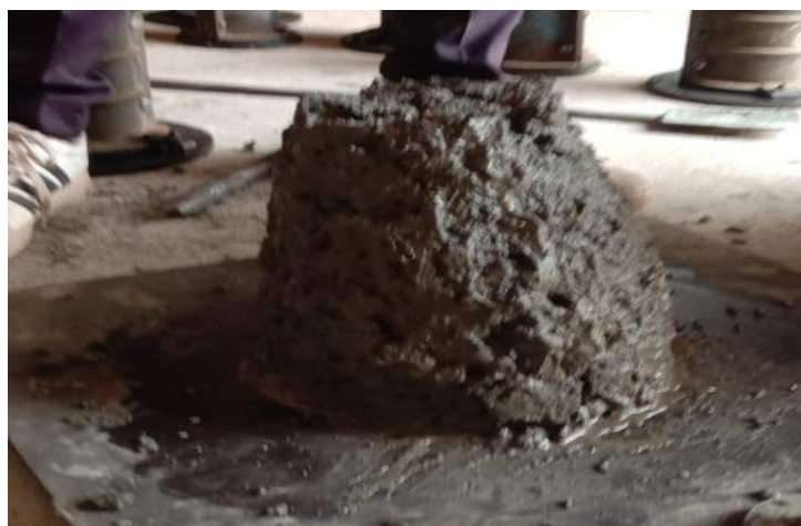
Fig.2 Slump cone test
