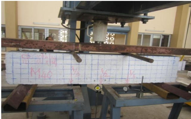
Fig 5.3 Displacement measurement of concrete beam
