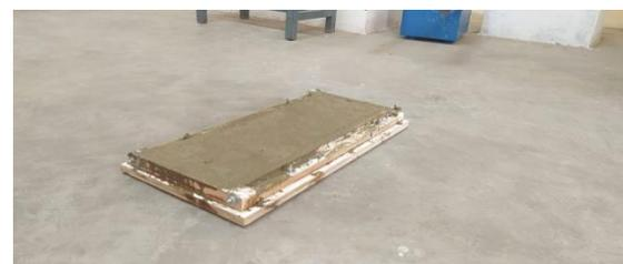
Fig.2.1 casting of ECC concrete in slab
