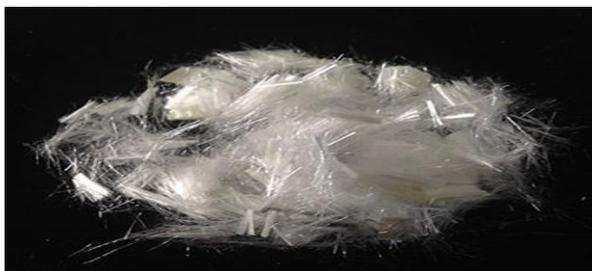
Fig.1.1 PVA Fibre
