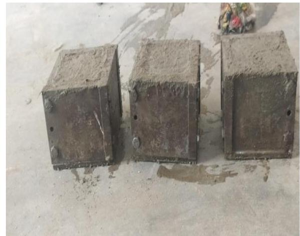
Fig.2. Casting of ECC concrete in cube.
