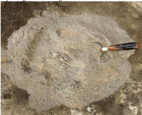
Fig.1. Mixing of ECC concrete.
