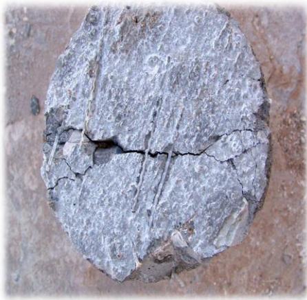
Fig.7 Shows Failure of fiber reinforced SCC
