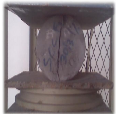
Fig.6 Split tensile test on cylinder
