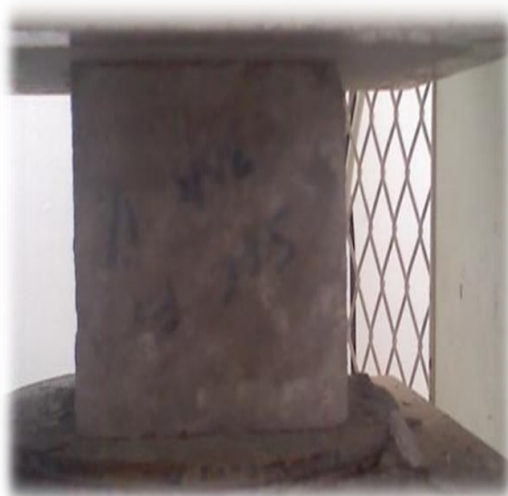
Fig.3 compression test on cube
