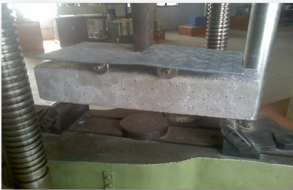
Fig.7 Shows Failure of fiber reinforced SCC
