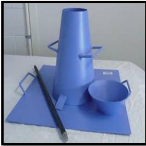
Fig. 5.4: Slump Cone Apparatus with Sketch
