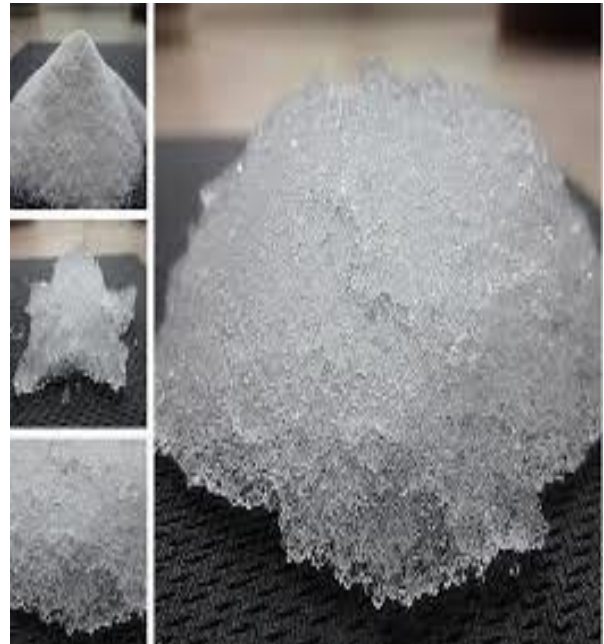
Fig.5.2: Powdered form of Super Absorbent Polymer (SAP)
