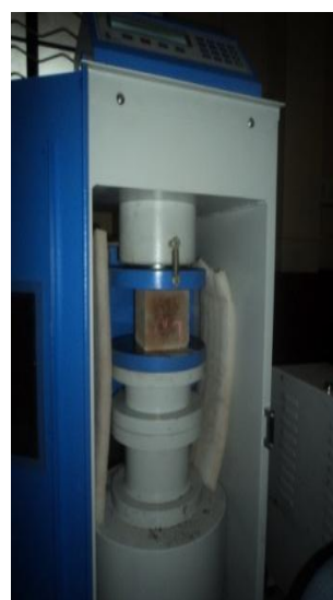
Fig 2: Compressive strength Test
