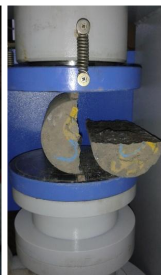
Fig 3: Split Tensile Strength Test
