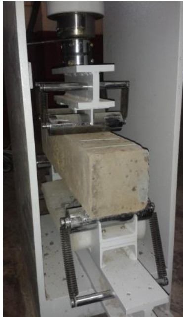
Fig 4: Flexural Strength Test
