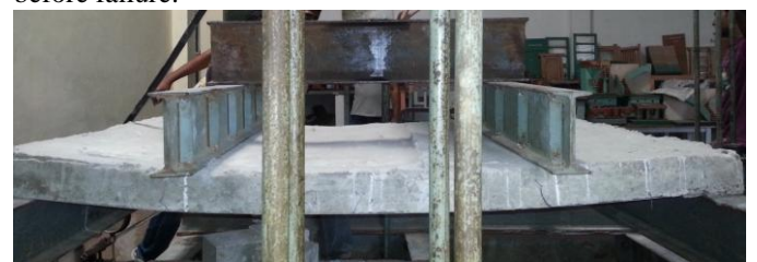
Fig.3 Failure pattern of composite slab with design mix concrete.
