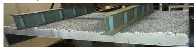
Fig.3 Failure pattern of composite slab with no fines concrete.
