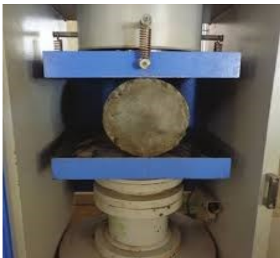
Figure 4: Cylinder Under Compression Testing Machine
