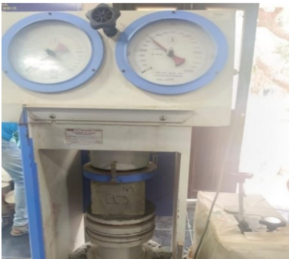
Figure 2: Cube Under Compression Testing Machine
