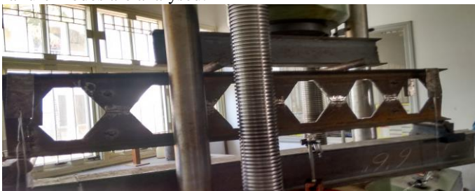
Figure 8 shows the loading arrangement of IC300 WOS
