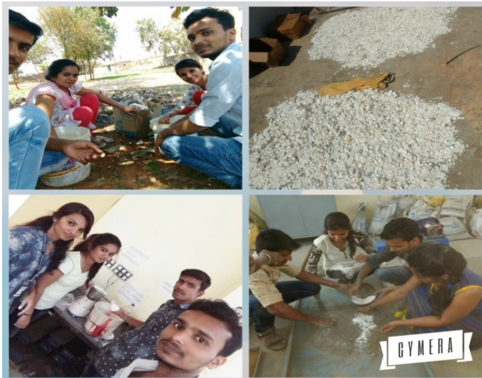
Fig2.Processing of eggshell waste(i)washing (ii)Air drying (iii) grinding & sieving (iv) Mixing.
