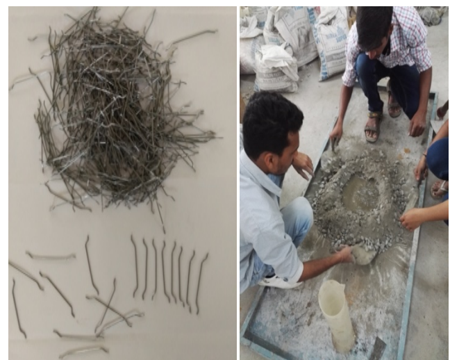
Fig 1. Steel Fibres along with mixing.
