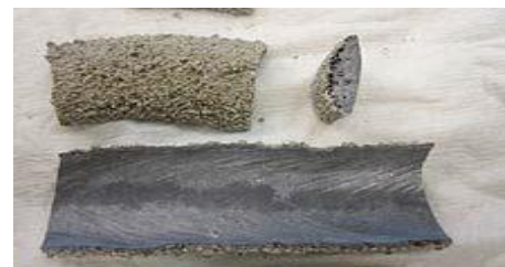
Fig 1.1 : submerged arc welding slag
