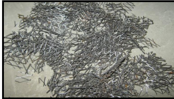
Figure (6): Steel Fibres used in Experiments of Stage (II).
