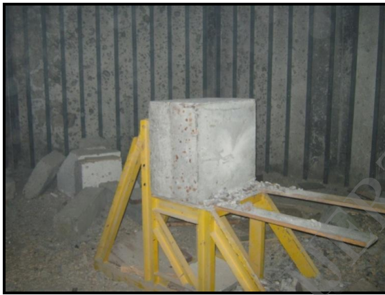
Figure (3-a): Steel mounting frame.
